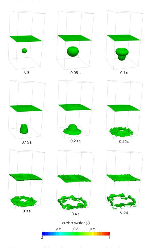
3D depth charge, alpha = 0.5 iso-surfaces, parallel simulation
